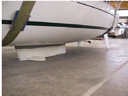
With the centerboard version it is possible for the boat to rest on the centerboard trunk and be balanced by the twin rudders when grounded during low tide (providing that it is sitting on a firm & stable bottom). Or when hauled out, the boat can be stored in this manner with a minimum of added support.
