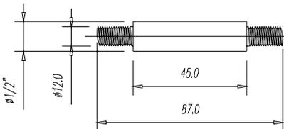
THREADED STEPPED PIN ATTACHES SWAGE EYE TO THE DOUBLE JAW TOGGLE & PROFURL LINK PLATES
