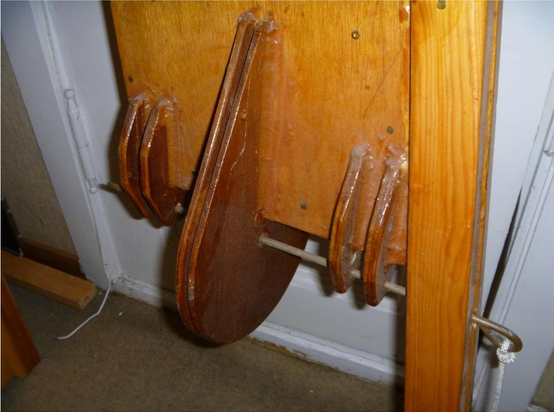
**Here the needle-type horizontal shaft can be seen. It was just held in place with a line.**
