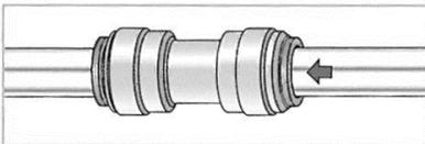
Push the tube into the fitting, to the tube stop.
