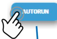
Gives you the option to run for a preset amount of time, or a preset volume of water to be produced. **If no tank switches are installed, and they have been disabled in the system settings, this is the only Operating Mode available.**
