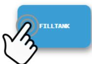
Runs your watermaker until the Tank Full switch closes, fresh water flushes the system, then goes into 'Auto Store' mode and the Flush Interval timer starts. *This is the default mode of operation.*
