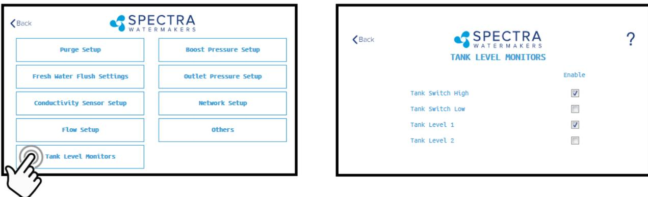
**Tank Setup** - Enable/disable tank sensors.
