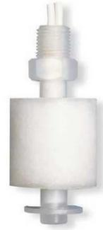
Drill and tap a 1/8" npt port into the top of the fresh water tank that is being filled by the watermaker. This can be installed on a tank access cover, or directly into the water tank. If installing on an access cover, be sure to leave a service loop on the float switch wiring to allow removal of the tank access cover.
