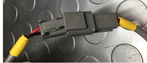
Connect the yellow boost pump connector from the bottom of the feed pump housing to the corresponding connector routed from the boost pump.
