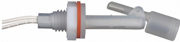
Installing the tank low float switch about 2/3rds down from the top of your water tank allows the Spectra Connect to run in Auto Fill mode; automatically filling your water tank, stopping itself, fresh water flushing, returning to Auto Store mode, and then turning itself on again to fill the tank when the water level drops below the Tank Low Switch with no additional user commands.
