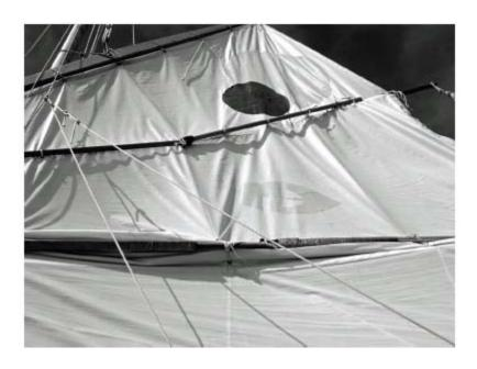
Mingming's jury rig, mainly boat hooks and gaffer tape. We sailed well over two thousand miles under these patched up battens.
