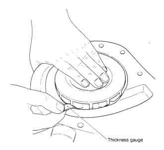
Measuring clearance between impeller and pump body bracket.
