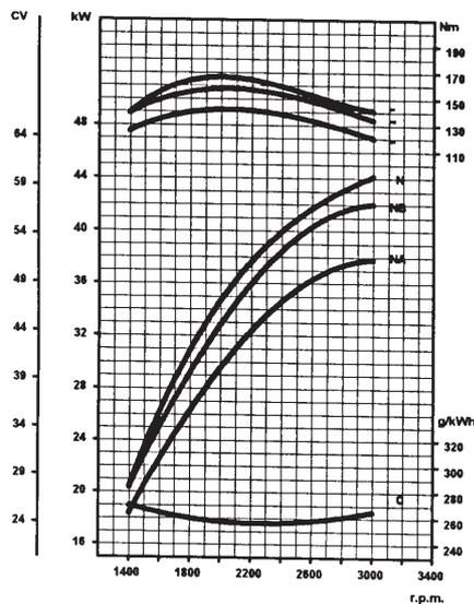
**N (80/1269/CEE - ISO 1585) AUTOMOTIVE RATING:** intermittent operation with variable speed and variable load.
