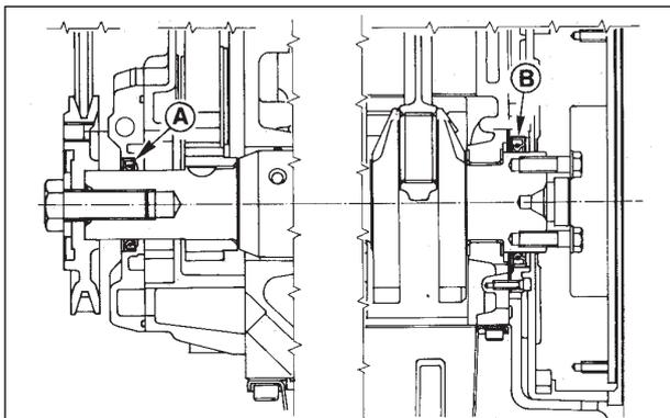
**Crankshaft front and rear oil seal**
