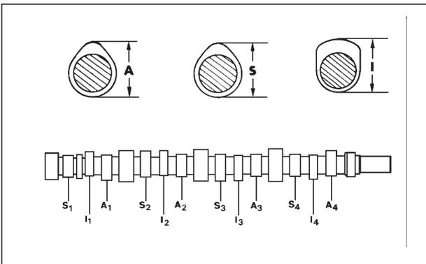
**Intake, exhaust and injection cam height for models LDW 2004, LDW 2004/T**
