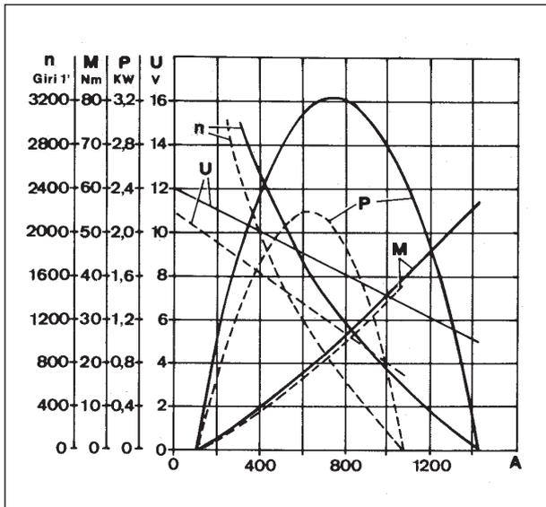
**Characteristic curves for starting motor type Bosch EV 12V 2.2 kW**
