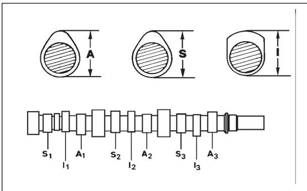
**Intake, exhaust and injection cam height for model LDW 1503**
