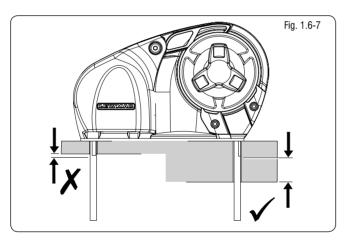
O DO NOT use a permanent adhesive/sealant, e.g., 5200 to the base of the windlass, any mounting pad or around the studs.
