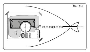
Using a 10 mm (3/8") diameter drill, make the three holes for the mounting studs and two for the motor wires. With a 76 mm (3") diameter hole saw, make the hole for the rode to pass through. When all the holes have been made, remove the template. To help avoid water absorption by the deck, apply an appropriate marine sealant to the freshly cut hole edges.
