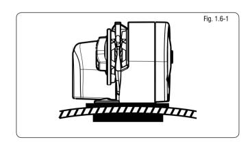
· Place the windlass on the deck and decide upon a position for it with reference to the vessel's bow roller (Fig. 1.6-2) and the chain locker below. Rode lead from the roller should ideally be fed horizontally back to the top of the gypsy and along its centerline (Fig. 1.6-3).
