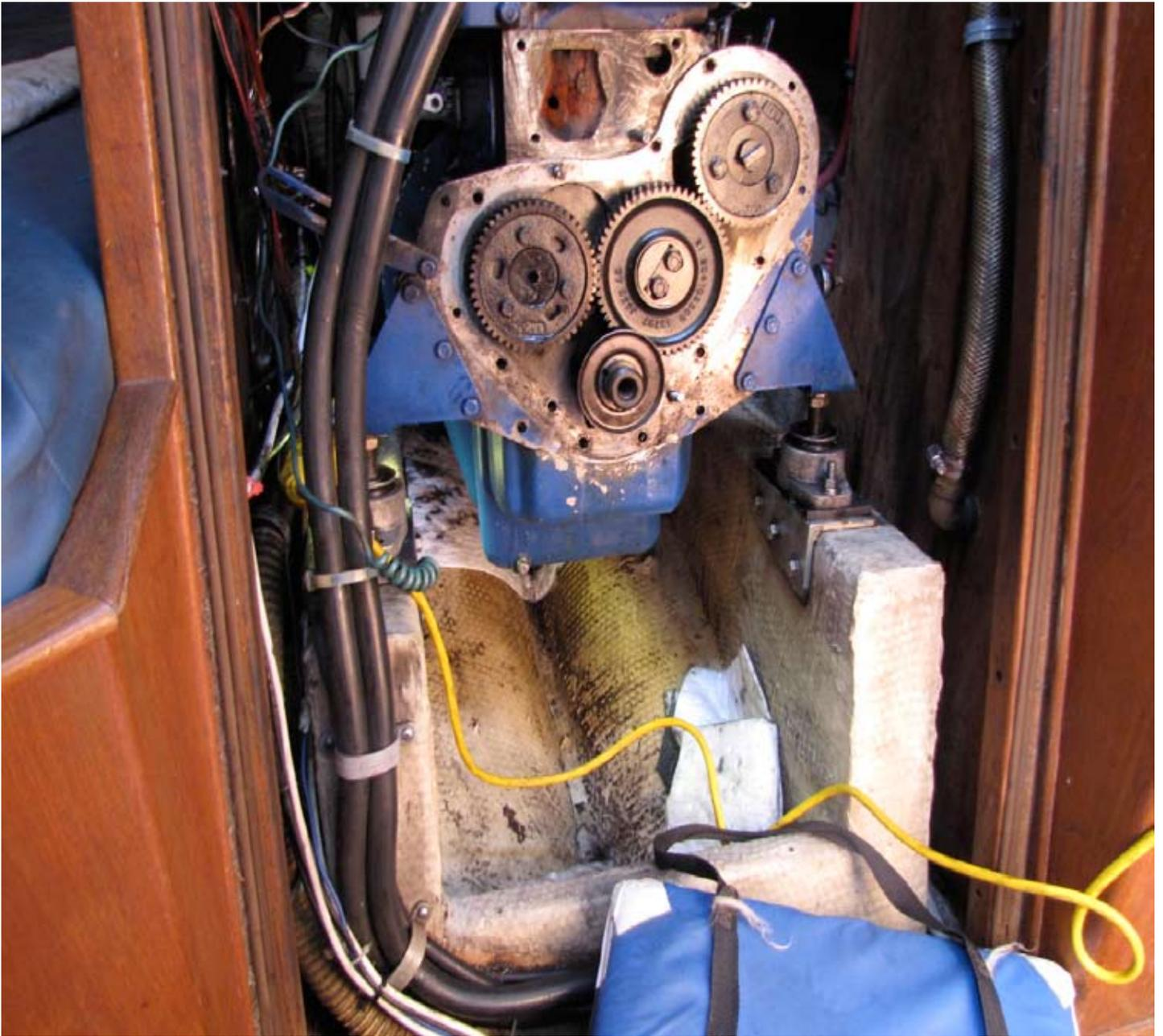
**Remove fresh water pump and timing case. Clean surfaces**
