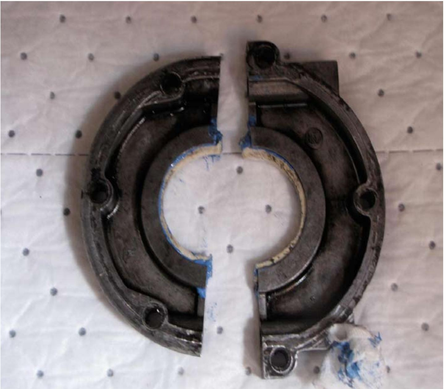
**two halves of oil seal mount ready for positioning**
