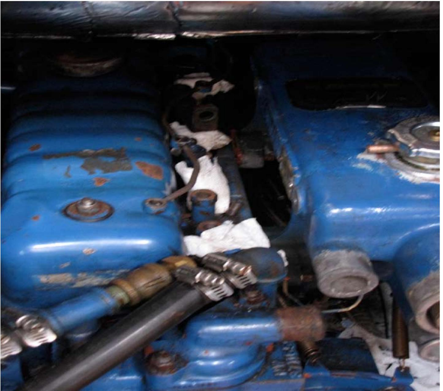
**Remove injectors and heat exchanger (right). Remove all hoses**
