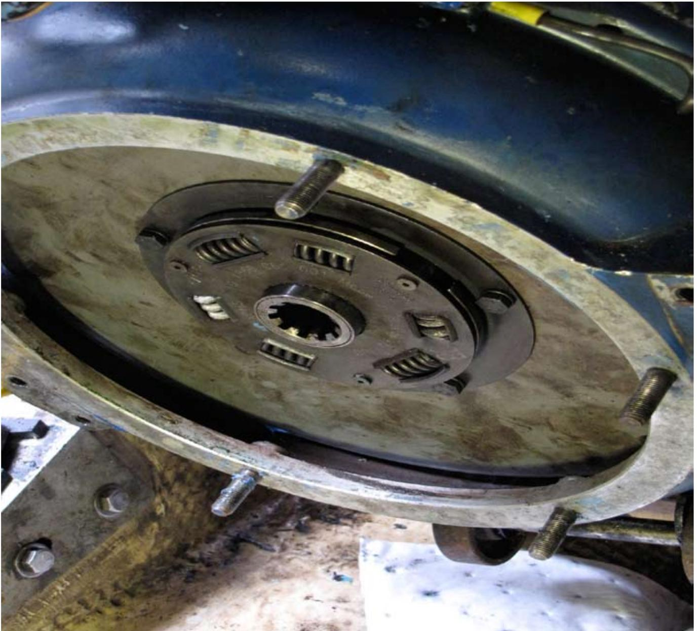
**Coupler is attached by five small bolts to flywheel**
