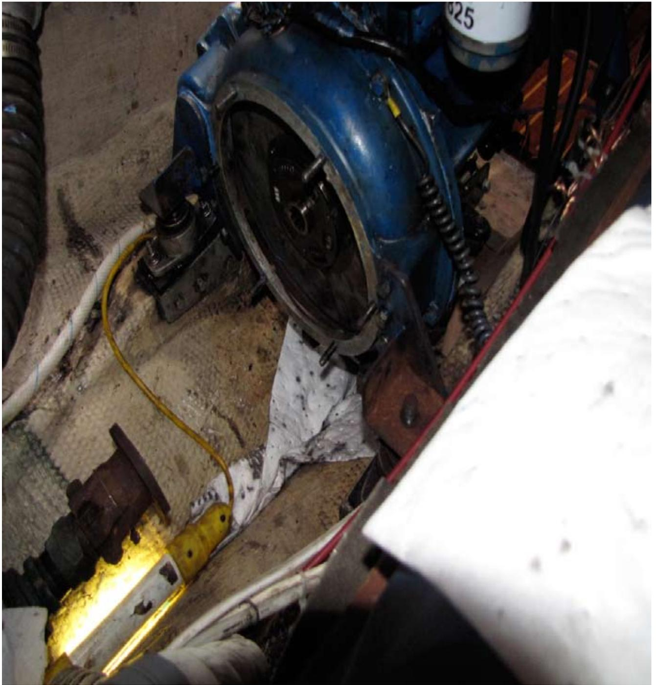
**Gear box removed, showing bell housing and coupler.**
