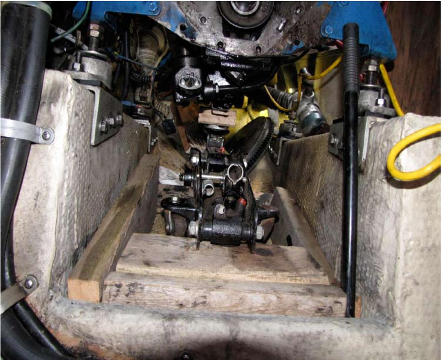
**It took me a bit of time to work out how to jack up the engine and at the same time maintain stability and engine alignment. One has to jack up the engine in order to take the weight off the rear engine mounts so that the flywheel bell housing can be removed.**
