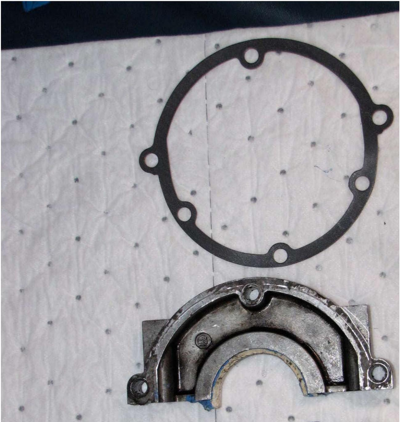
**Oil seal gasket and upper half of oil seal. The oil seal gasket is positioned between the oil seal housing and the rear engine casting. First place the gasket loosely on shaft, then join the oil seal half mounts and bolt together around shaft. Then bolt the oil seal housing to back of engine with the oil seal gasket in the correct position.**
