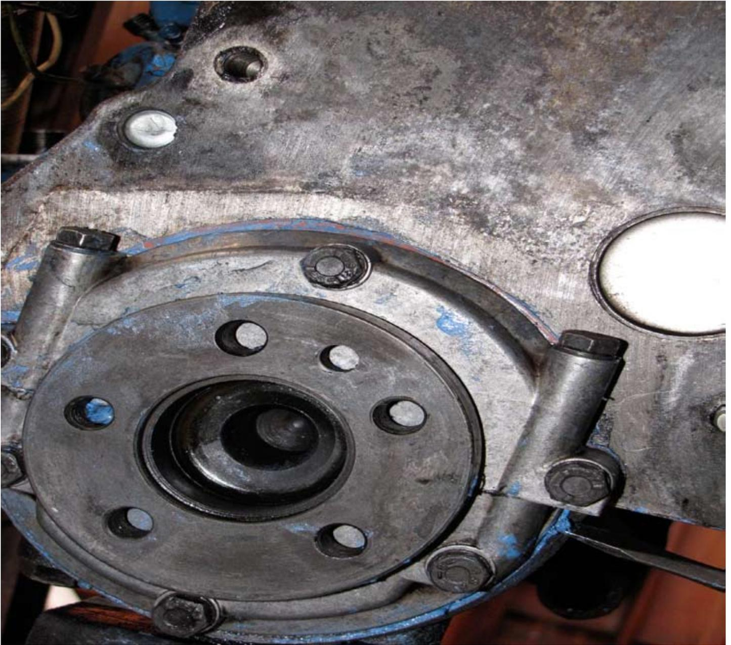
**New oil seal and mount bolted to engine casting; Face view**
