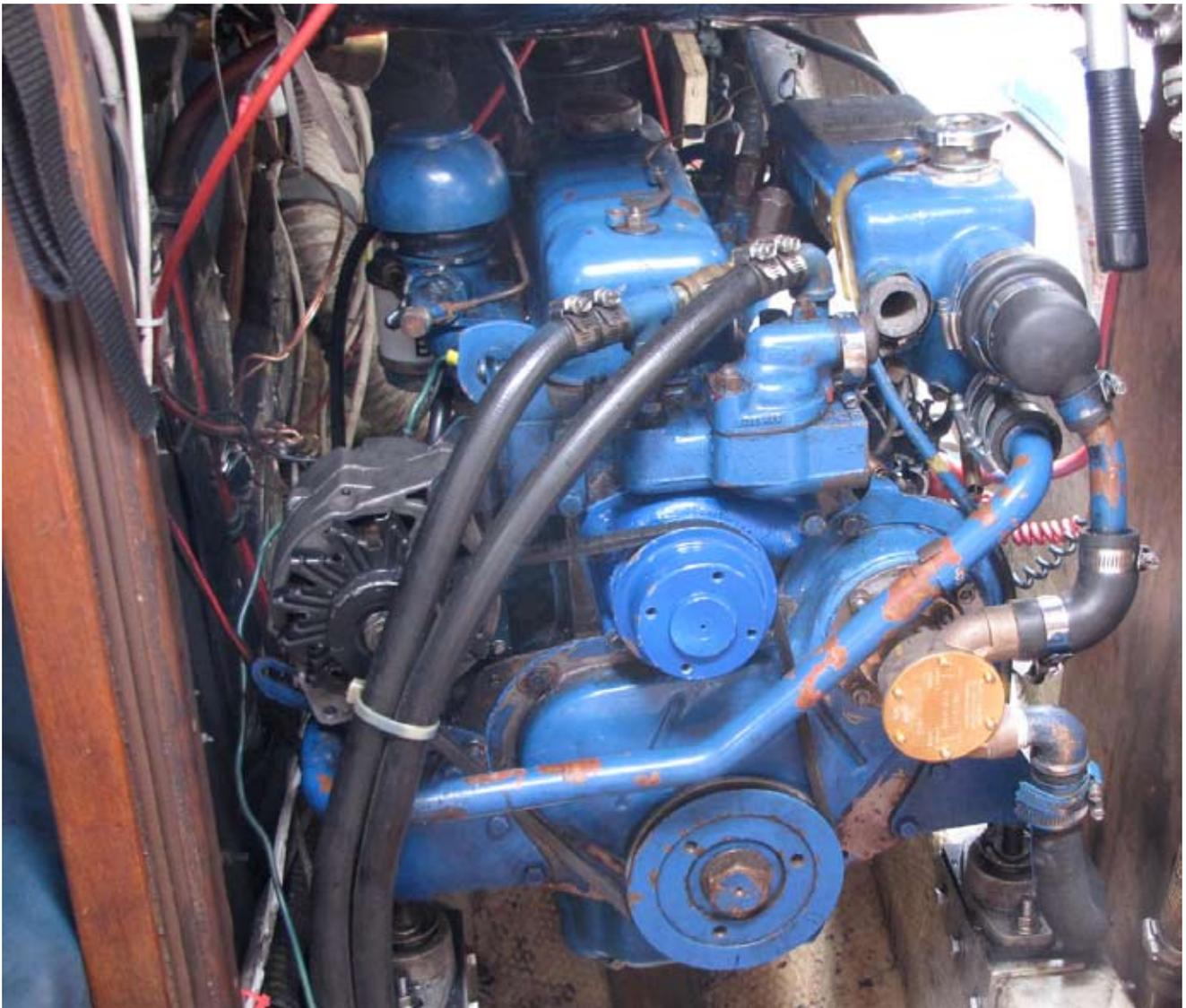
**Just about finished. Front view: new freshwater and raw water pumps, new hoses and best of all not a single drop of leaking oil.**
