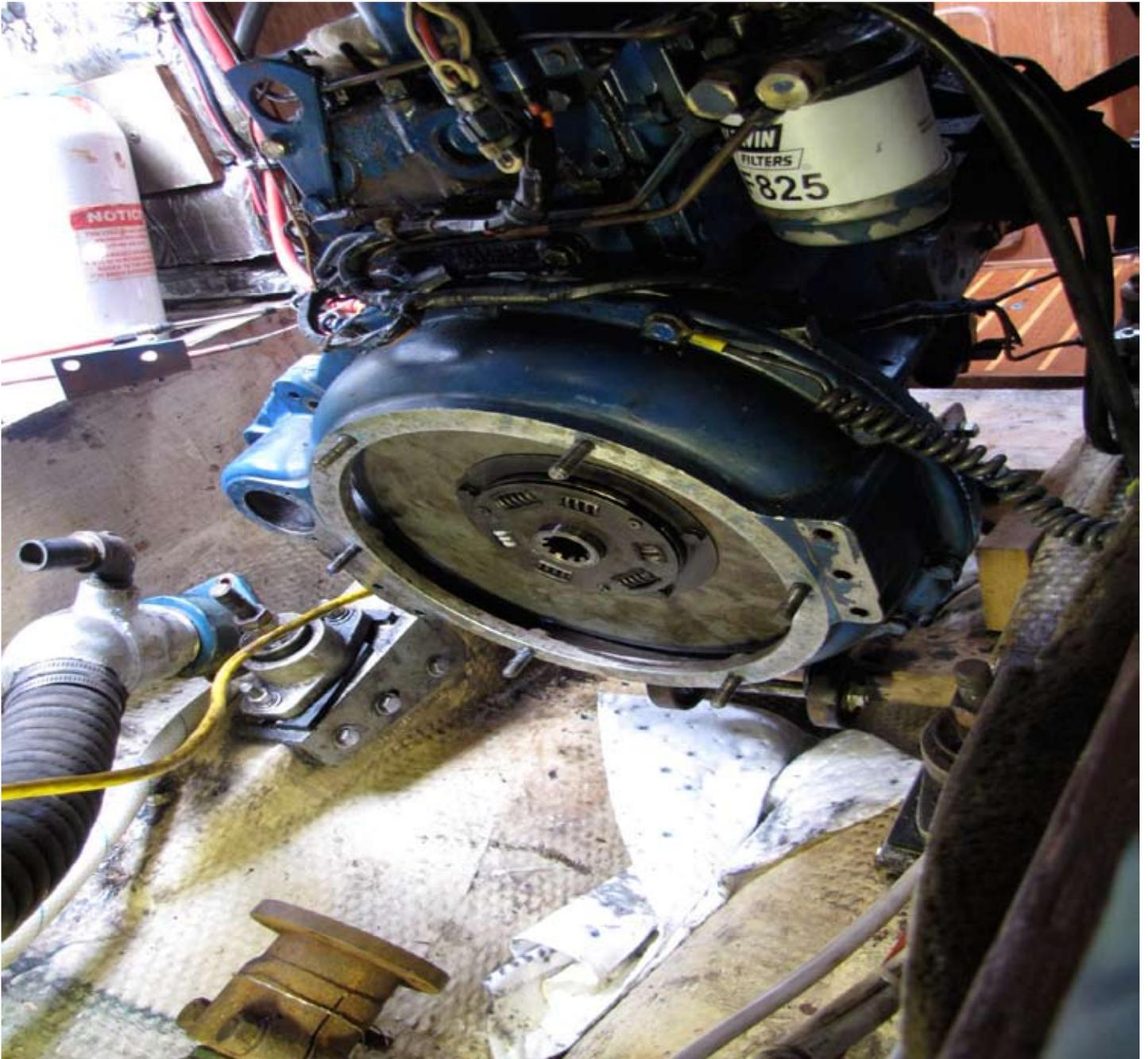
**Both brackets removed leaving bell housing and engine supported by jack**
