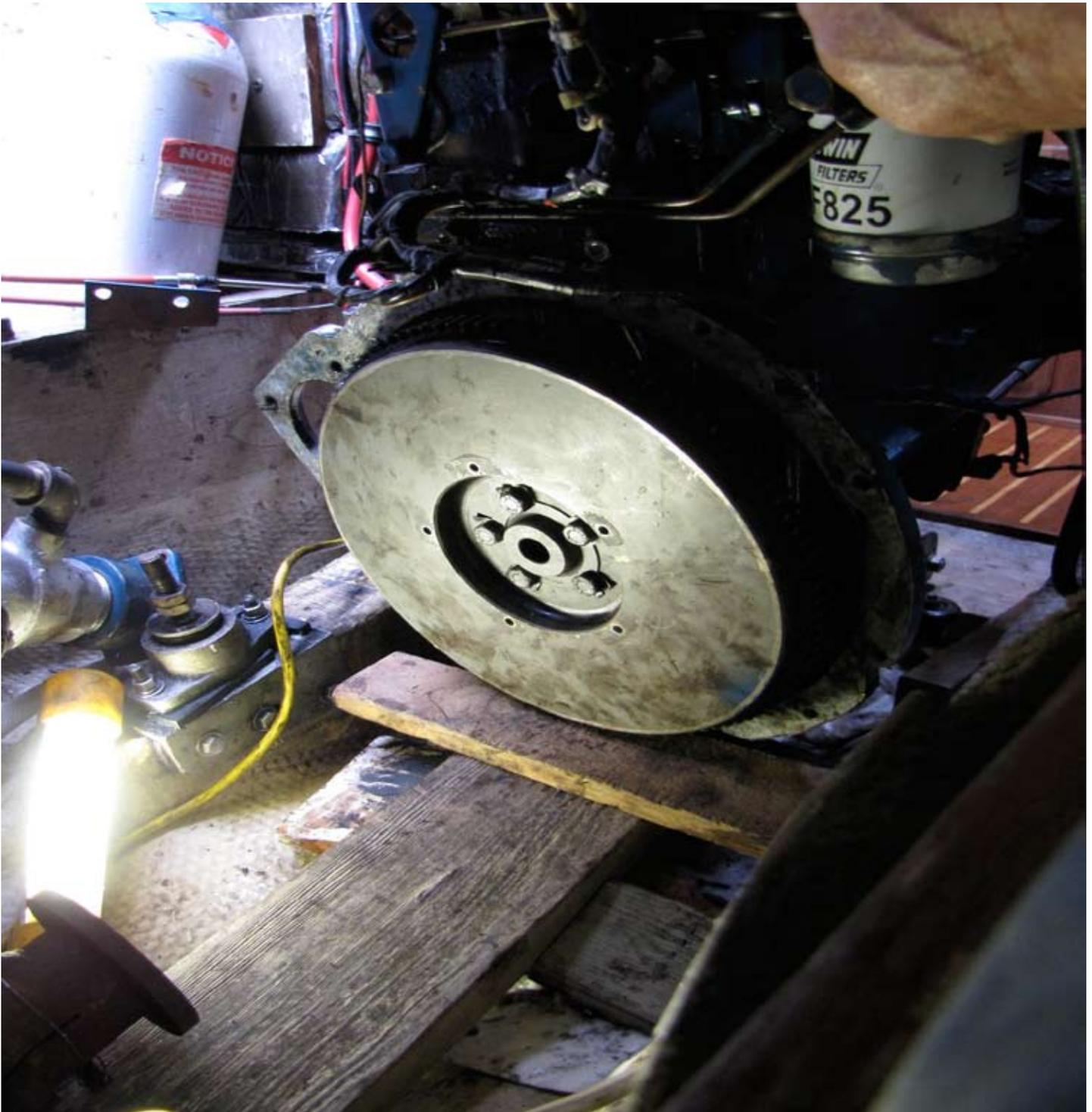
**Remove bellhousing - showing flywheel. Note the wood under flywheel was placed there to assist in the attachment of the flywheel when putting everything together again. The flywheel is heavy (30lbs) - not easy to pick up and position by oneself - a helper would be handy!**
