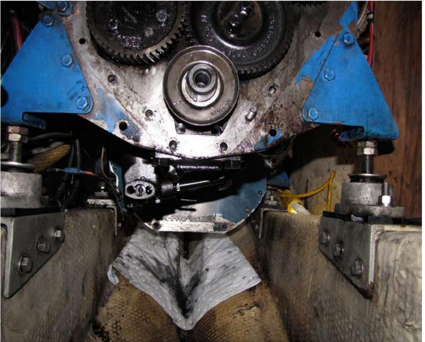
**In order to use the jack to jack up engine I removed crankcase oil pan oil filter**
