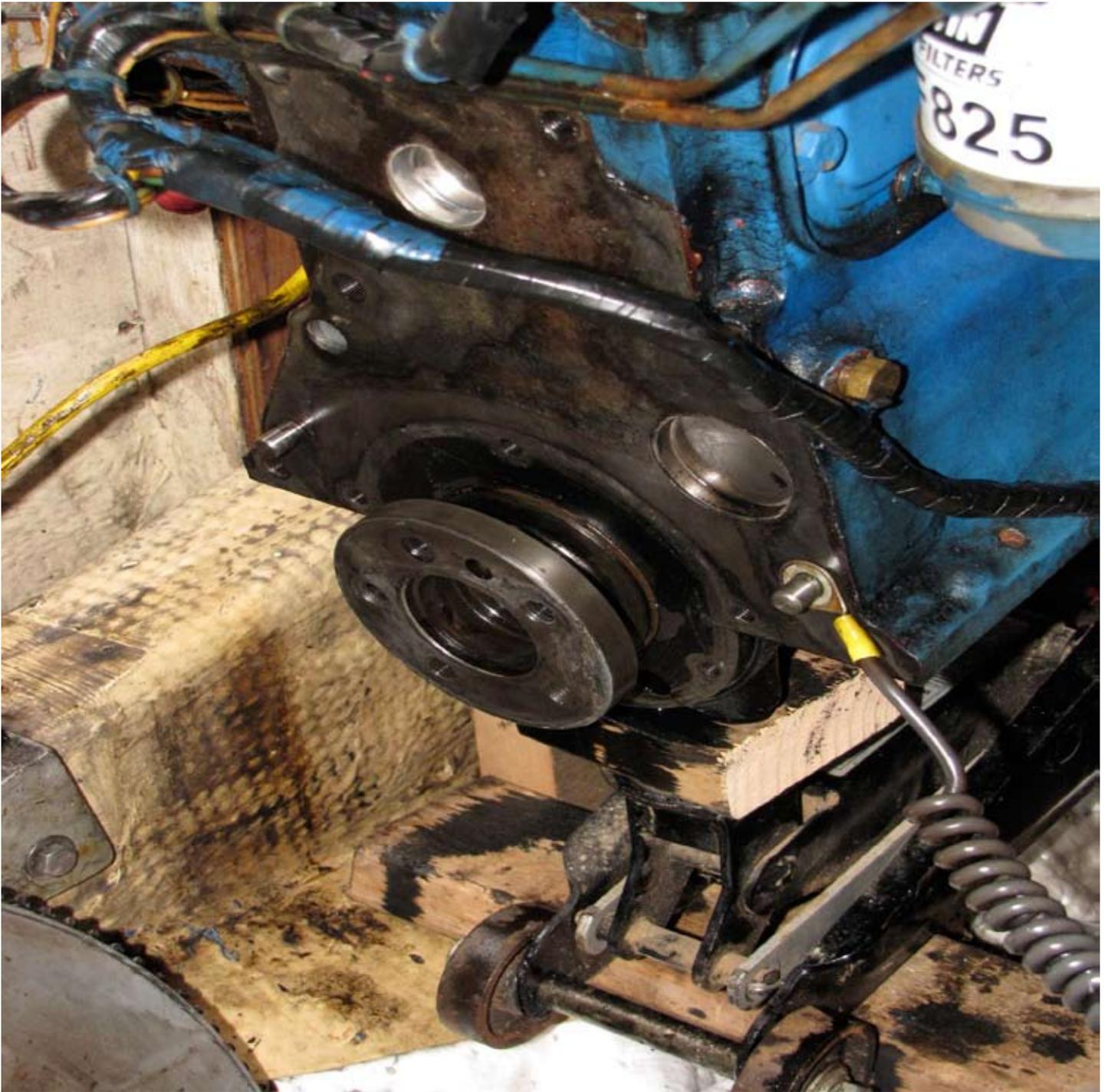
**engine shaft coupler flange. The groove immediately behind flange is where the oil seal housing fits. Note how I have positioned the jack**
