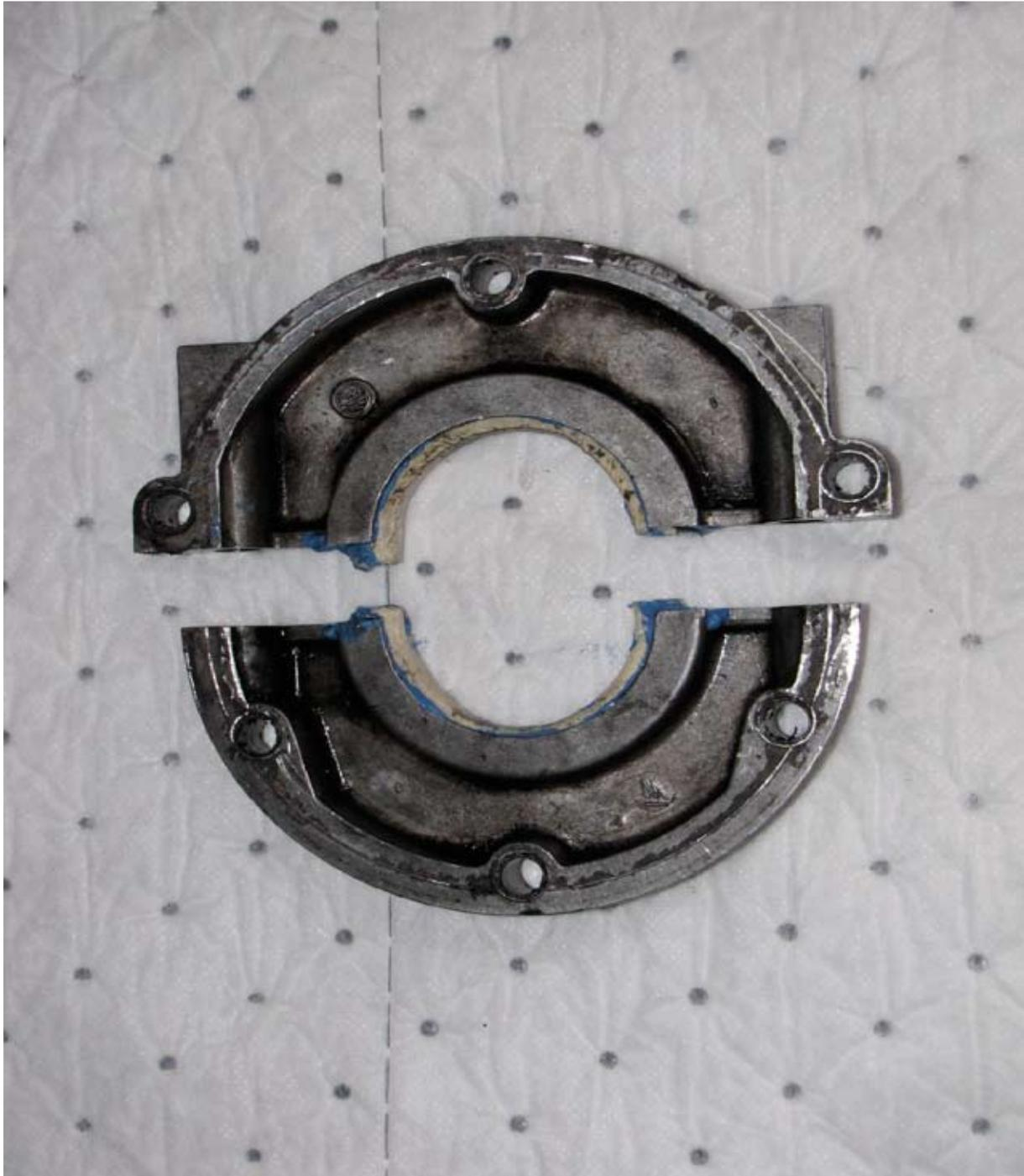
oil seal mount with near oil seal fitted. It is a good idea to soak the oil seal in oil for 24 hours before fitting.
