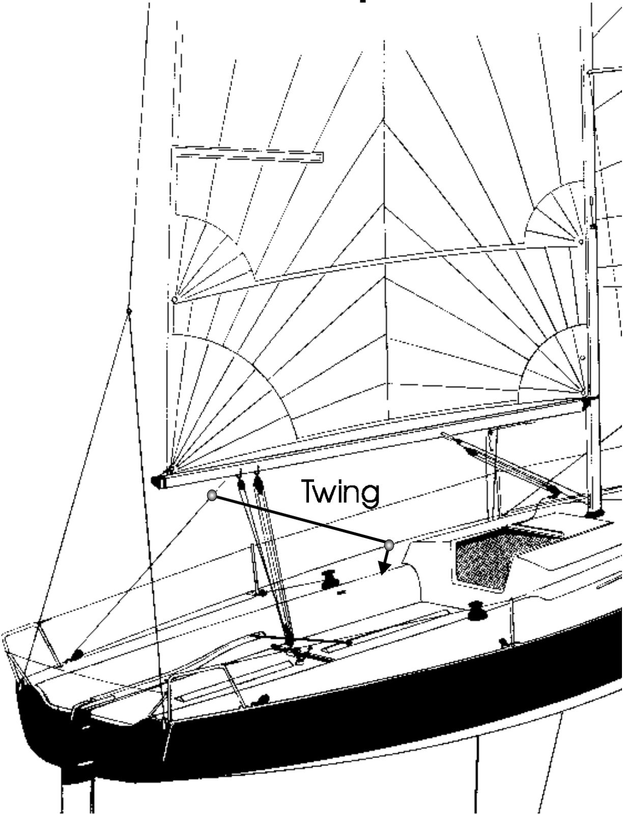
broader angles, is to "twing," or move the sheet lead forward. (see diagram). This keeps the clew from rising up and dumping off the leech, making the sail more symmetrical and powerful.
