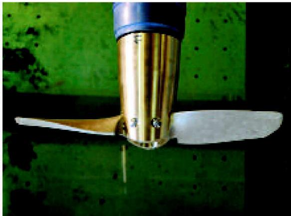
The majority of propellers tested were fitted with a zinc anode. The "Maxprop" (l) gives in addition a more streamlined transition between boss and Sail drive. Allpa (r) without anode
