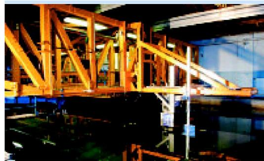
The giant towing carriage travelled at up to eight knots above the test tank
