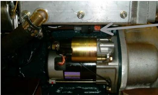
*FUSE (If located by starter motor, usually it is positioned above flywheel housing at rear of engine)*
