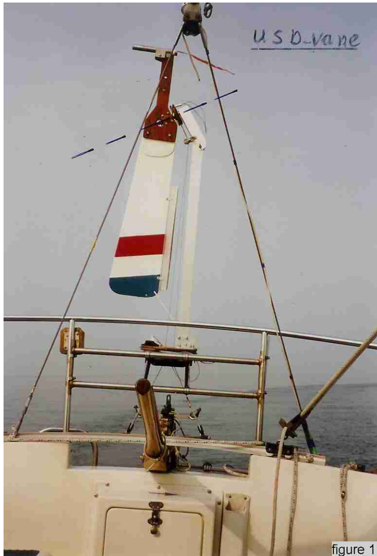
Figure 11: The USD windvane concept offers construction-inherent adaption to heel and needed steering force. V-shaped tabs at the trailing edge of the vane yield maximum output power.
