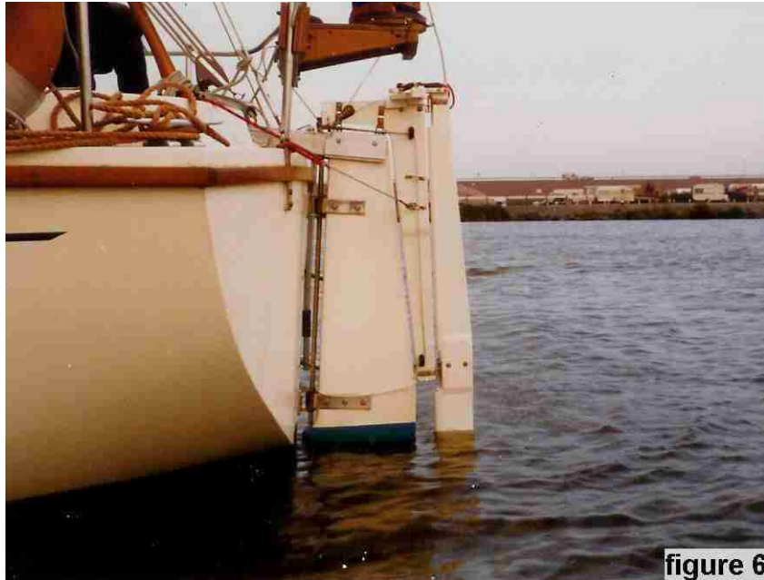
figure 6. The prototype of oar and oar carrier made from plywood (5 years in use)
