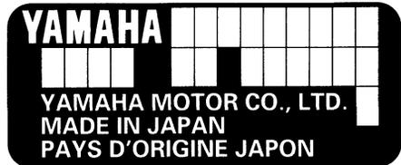
The outboard motor serial number is stamped on the label attached to the port side of the clamp-bracket. (2-hp model: attached the upper part of the swivel bracket.)
