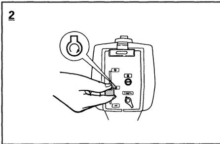
5) Place the throttle-control lever/grip in the "START" position.
