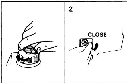
2) After stopping the engine, tighten the air vent screw and set the fuel cock lever / knob to the closed position.
