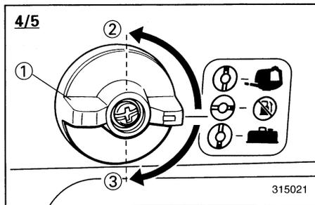
② "OPEN" position for the built-in tank
