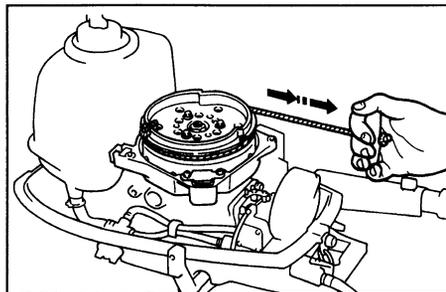
5) To start the engine with emergency starter rope, insert the knotted end of the rope into the notch in the flywheel rotor and wind the rope several turns clockwise. Then, give a strong pull straight out to crank the engine. Repeat if necessary.
