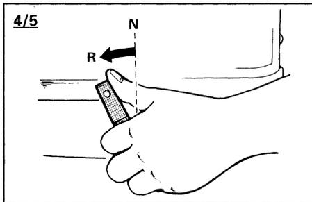
2) Turn the gear shift lever quickly and firmly from Neutral to Reverse.
