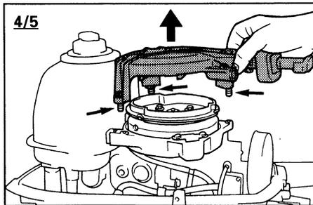
2) Remove the starter by removing the bolts.
