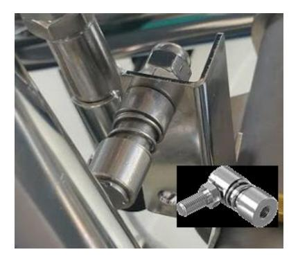
The ball joints are ¼"-28 threaded on both ends. When securing them it is highly recommended that Locktite thread locker be used. An alternative would be 3M 5200.
