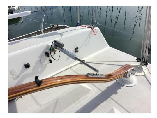
The Pelagic is Capable of Driving Hydraulics and a Variety of Linear Motors for Tiller or Quadrant
