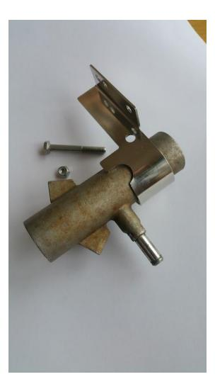
Attaching the WV pinion bracket. Slide It onto the pinion gear then tighten the bolt and nut combination. The bracket locks onto the pinion gear and the wind link arm.
