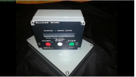
Original model: The USB connector is Exposed by removing the 4 screws On the front panel and then removing the circuit board with the 3 screws holding it in place.
