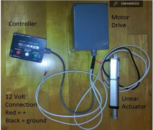
Actuator shown is for windvane control.
