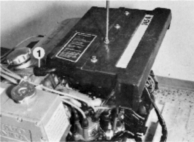
3. Remove the alternator, drive belt, cable harness, ignition coil, main fuse, starter motor, ignition cables and distributor. NOTE! Mark the cables before they are removed.
