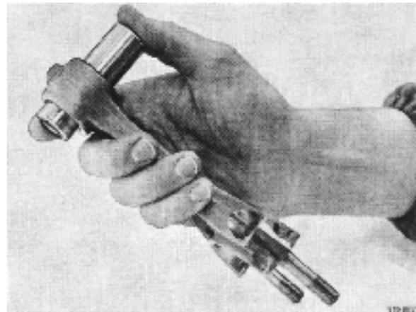
76. Check the connecting rods for straightness, torsion and possible s-bends. Use a connecting rod straightener. Nuts and screws are to be replaced when overhauling.
