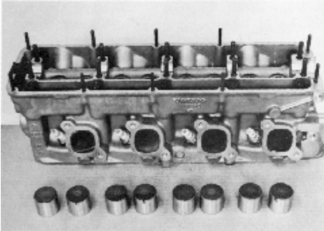
39. Remove the rubber ring, collets, upper washers, springs, lower washers and valves. Then remove the valve seals from the inlet valve guides. Clean all the parts. Remove carbon deposits from the combustion chamber and the valves.
