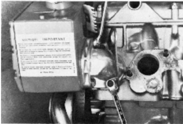
7. Remove the cap and lift out the strainer (1) from the heat exchanger. Then pull up the rubber ring's tongue (2). The tongue is marked "UP". The cover (3) is now loose and can be lifted up. (Not on AQ125.)
