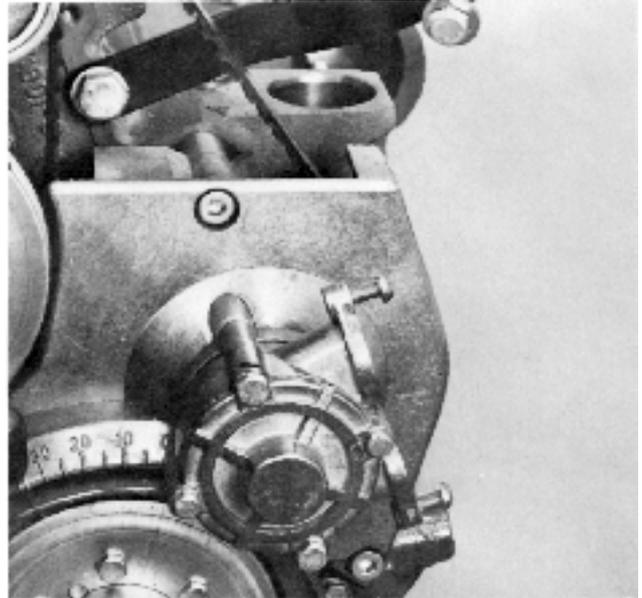
14. AQ145. If the oil cooler's channels are to be cleaned when the exhaust pipe is fitted on the engine the cooling water pipes (1) and (2) must be removed. Undo the oil cooler's screw (3) and remove the lower cover. The oil filter is then removed and the centre nut (4) is loosened so that the oil cooler can be turned to a horizontal position. After this the insert's channels can be cleaned.
