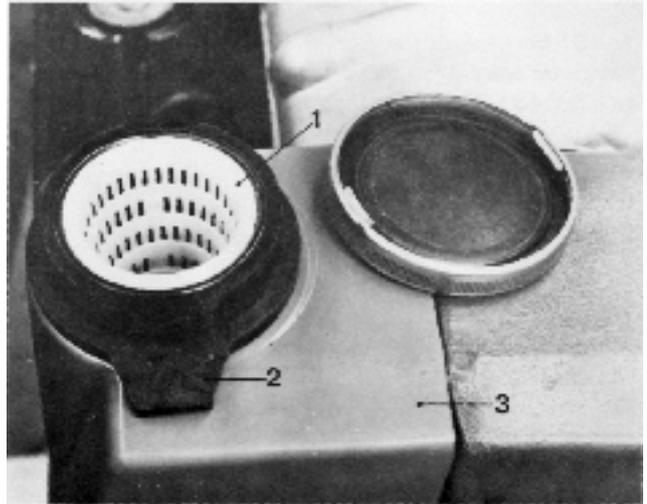
6. Remove and discard the O-ring (1) in the heat exchanger and if necessary, unscrew the holder (2) for the ignition cables. The holder is fixed with two guide pins.
