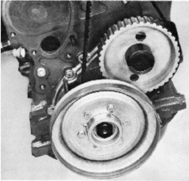
**133.** Fit a new O-ring on the cover for the oil pump drive.
