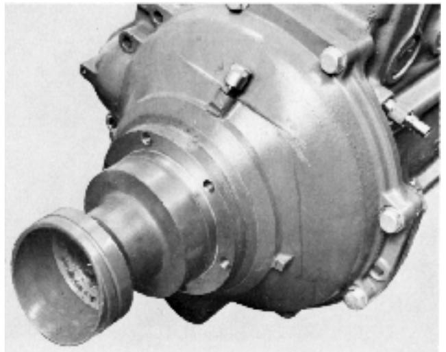
29. Remove the vibration damper's six screws. Spanner width 13 mm. Carefully remove the vibration damper from the three guide pins.
