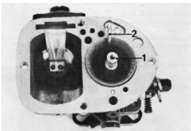
93. Rotate the throttle shaft (1) and press out the push rod (2) from the lever (3). Then rotate the push rod downwards and disassemble the check valve (4). Blow the check valve clean and the strainer. Clean and blow the carburetor and its ducts. Then re-fit the check valve and strainer. NOTE! Do not forget the copper washer. Rotate the throttle shaft somewhat and press the push rod into the lever.
