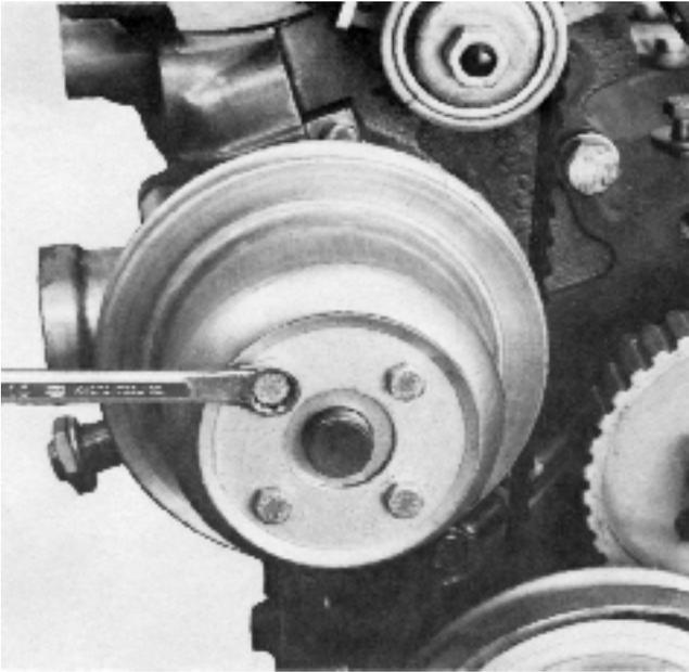
19. Remove the crankshaft pulley. Six screws. The spanner width is 10 mm.
