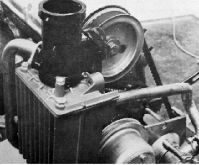
11. Remove the cooling water pipe between the oil cooler and the exhaust pipe. Not on AQ125. Then remove the exhaust pipe.
