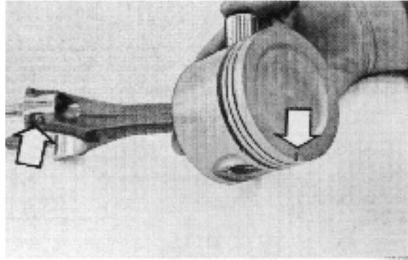
100. Fit the piston rings with piston ring pliers. The piston rings are to be fitted as shown in the picture. The upper ring is chromium-plated. The lower compression ring is marked "TOP". Turn the piston ring so that the gaps are at an angle of 120° from each other.
