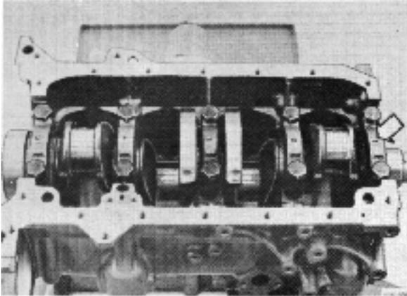
99. Refit the pistons and the connecting rods so that the marks on the pistons point forward in the engine when the figure marking on the connecting rods is turned towards the crankcase's starboard side (oil filter side). Fit the lock rings.
