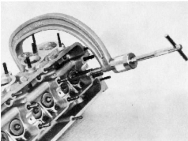
40. Grind the valves if necessary in a valve grinding machine. The angle is the same for both the exhaust and the inlet valves.
