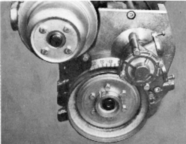
161. Fit a spacer ring and two sealing rings on the expansion tank's outgoing water pipe (1) and press in the tank's guide pin (2) and pipes in the heat exchanger. At the same time check that the support screw (3) has a plastic sleeve.
