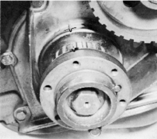
27. Remove the screws from the sealing flange. The flange is also tightened with two of the screws in the oil sump. Remove the flange plate and remove the seals. Use tool 999 5025 for the small seal and tool 999 5024 for the large seal.
