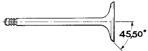
41. Mill or ream the valve seats. The angle is the same for the exhaust and inlet valve seats.
