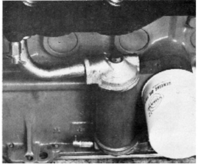
10. Remove the remaining three screws (X) on the heat exchanger and draw it to one side from the circulation pump.
