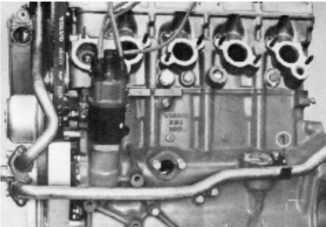
162. Place an O-ring (1) on the expansion tank and fit the thermostat (2). When necessary the opening temperature of the thermostat is checked by lowering it in hot water. At a temperature of 82°C (180°F) it must begin to open and must be fully open at 92°C (198°F). Check that the rubber seal (3) is not damaged when the thermostat is fitted. NOTE! The forward lifting eye is fitted on the thermostat housing.
