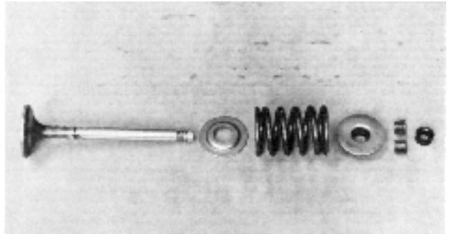
38. Remove the valves. Use valve spring compressor 884 580.
