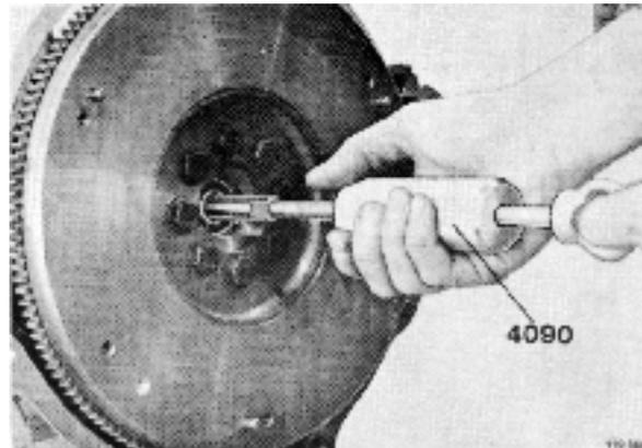
55. Remove the sealing flange. NOTE! Two screws from the sump must also be removed.
