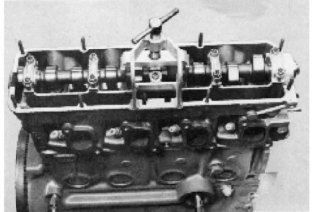
114. Oil and fit the last bearing cap. Then tighten all the nuts with a torque wrench. The tightening torque is 20 Nm (2.0 kpm) (14.7 lbf. ft.).
