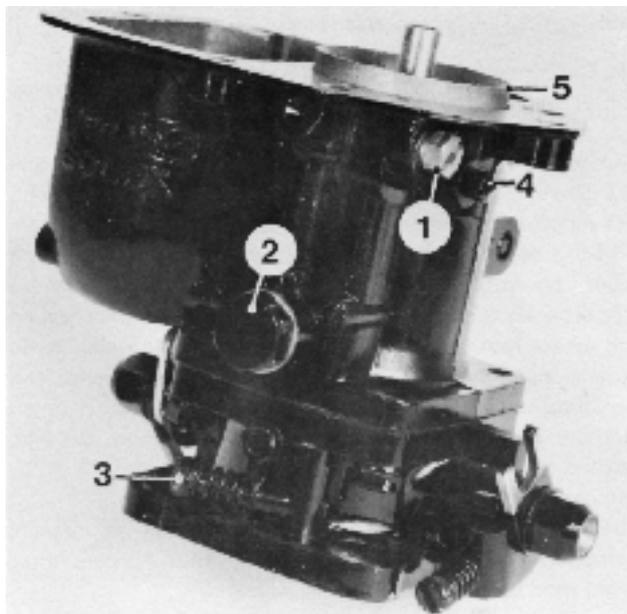
91. Lift out the float tube and check that it is tight. If the float is not tight the float level will be wrong. Unscrew the emulsifying jet (1) and the acceleration jet (2). NOTE! The gasket. Check and clean with compressed air. Replace worn or damaged parts if necessary.
