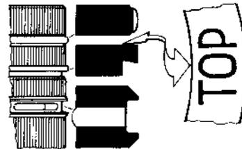
98. Check the axial clearance which is 0.037–0.147 mm (0.0014–0.0058").
