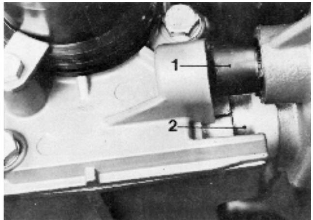
9. AQ145. Remove the cooling water pipes between the seawater pump and the heat exchanger and between the heat exchanger and the oil cooler. (Between the heat exchanger and the exhaust pipe on AQ125.)
