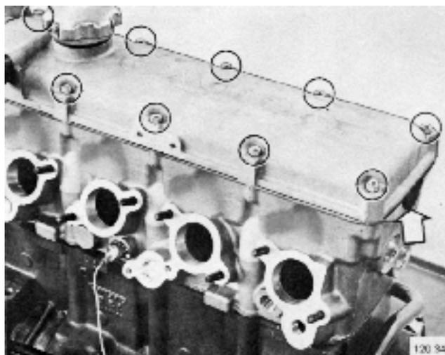
33. Remove the centre camshaft bearing cap. Spanner width 1/2". There are spring washers under the nuts. When necessary use a chisel or similar tool against the lug as shown by the arrow.
