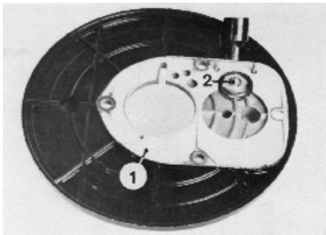
92. Disassemble the idling jet (1) and holder (2) for the main jet. Unscrew the jet from the holder. Blow the jets clean and replace if necessary. Unscrew the mixing screw (3) and blow clean the duct. Screw (4) locks tight the air cone (5).
