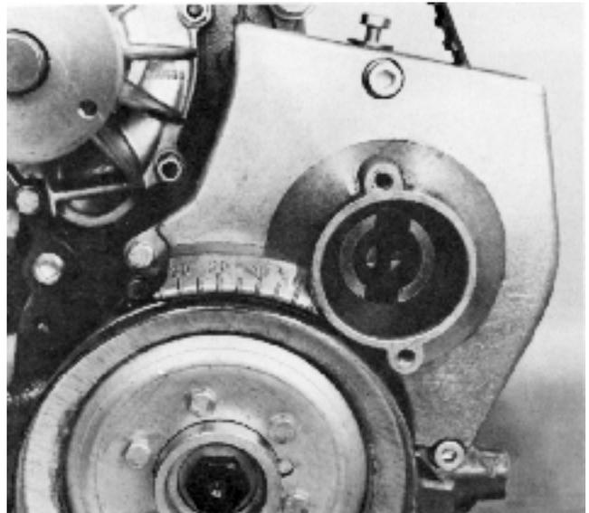
17. Remove the circulation pump's pulley. The spanner width is 10 mm.
