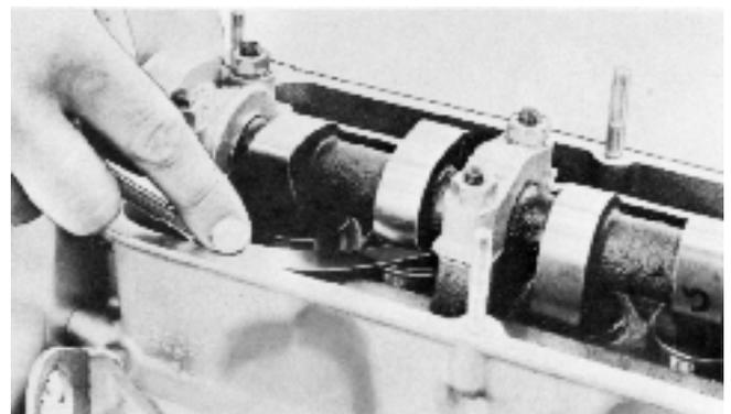
**139.** If the clearance is incorrect the adjustment shims are to be changed as follows: Turn the valve pusher so that the groove is at right angles to the camshaft's length.
