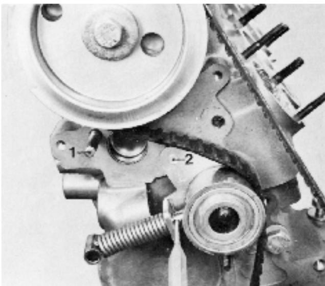
24. Remove the pulley from the camshaft. Use counterforce 999 5034. Remove the pulley by hand. Check that the outer and the inner guide plate's edges are not damaged so that these in turn can damage the belt.
