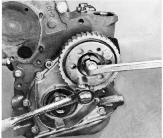
22. Remove the belt tensioner from the shaft (1). The belt tensioner's guide pin 2 is now free after which the belt tensioner is twisted and removed. Then remove the belt. The shaft (1) can be replaced by unscrewing it from the cylinder head. The timing belt is to be changed if the cord re-inforcement and the rubber are beginning to separate or if the tread on the timing belt is worn. The timing belt is to be changed every five hundred hours.
