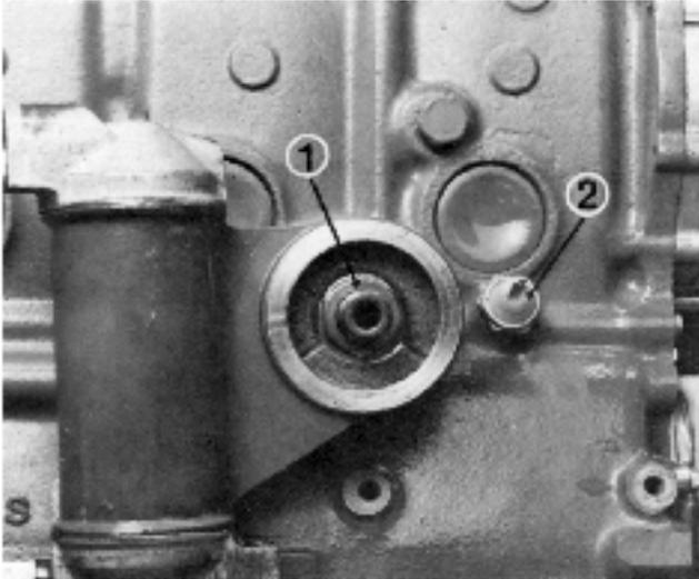
15. Remove the saltwater pump and the generator's tensioning bracket. The spanner width for the saltwater pump is 10 mm. The other screws which hold the cover have a spanner width of 8 mm. Check the impeller, the key and the packing on the pump's front side plus the sealing ring on the pump's rear side. Clean the pump and replace damaged parts.
