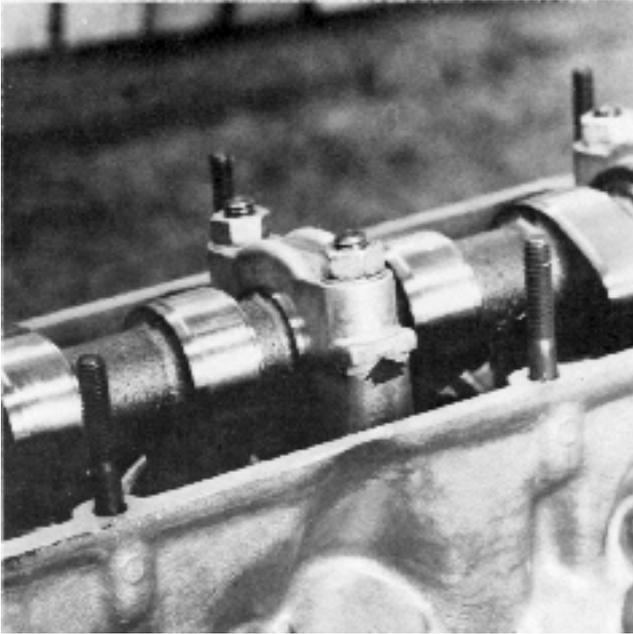
35. Remove the seal (1) from the camshaft. Then undo the tool spindle and release the camshaft. Remove the tool and lift out the camshaft.
