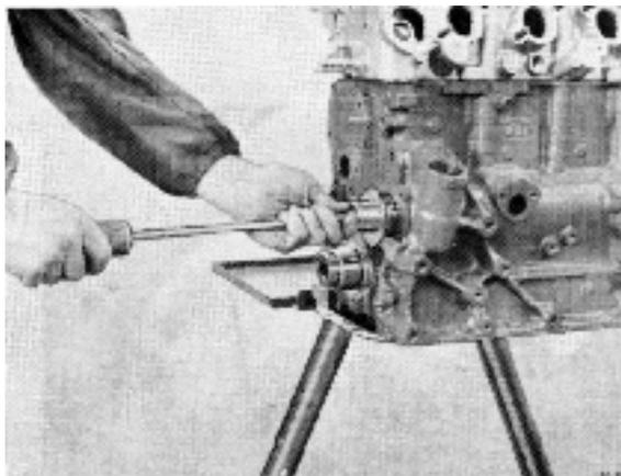
30. Remove the cover and the bracket for the oil pump drive. Then lift up the oil pump drive.
