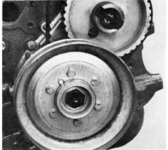
18. Remove the circulation pump. The spanner width is 10 mm. There are four screws and two nuts with washers. Discard the plain packing and the rubber seal. NOTE! The pump is to be changed as a complete unit if it has been damaged.
