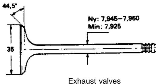
IMPORTANT! The valves have a stellite coating. Therefore, they are not to be cut or ground but only lapped into the seat.
