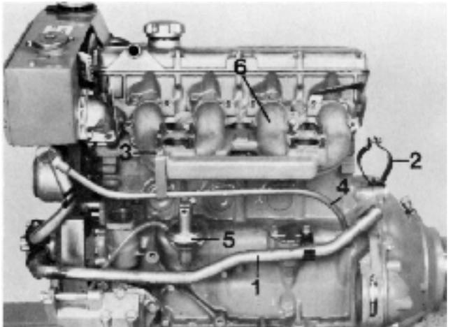
5. Remove the thermostat housing and lift out the thermostat.
