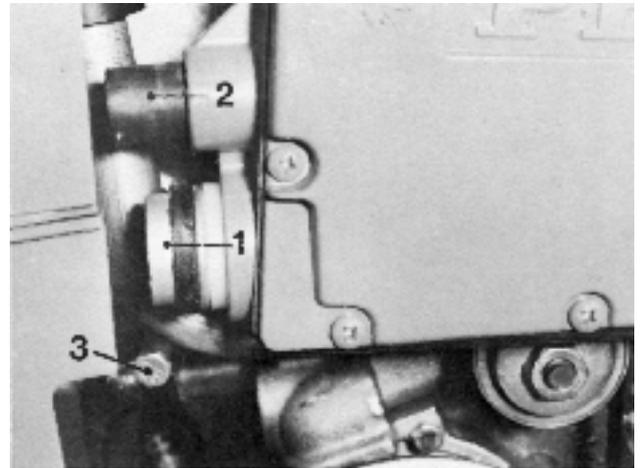
160. Fit the ingoing and outgoing cooling water pipes to the salt water pump and press the ingoing pipe into the bracket (1).
