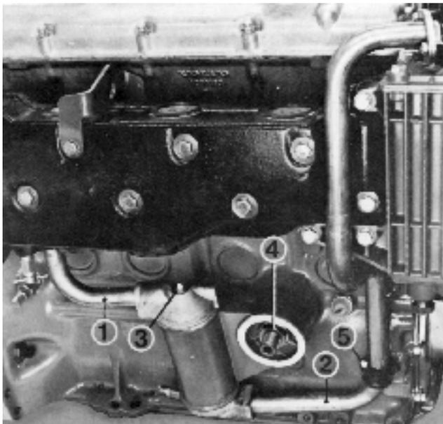
16. Undo the cover's two hexagonal socket screws (6 mm key) and hexagonal screw (spanner width 10 mm). NOTE! The cover's upper fixture is fitted with a guide which means that the cover must be withdrawn a few millimetres before it is free.
