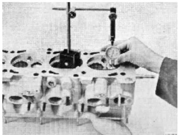
45. Replace the camshaft in the cylinder head and check the axial play which is 0.1–0.4 mm (0.004–0.016").
