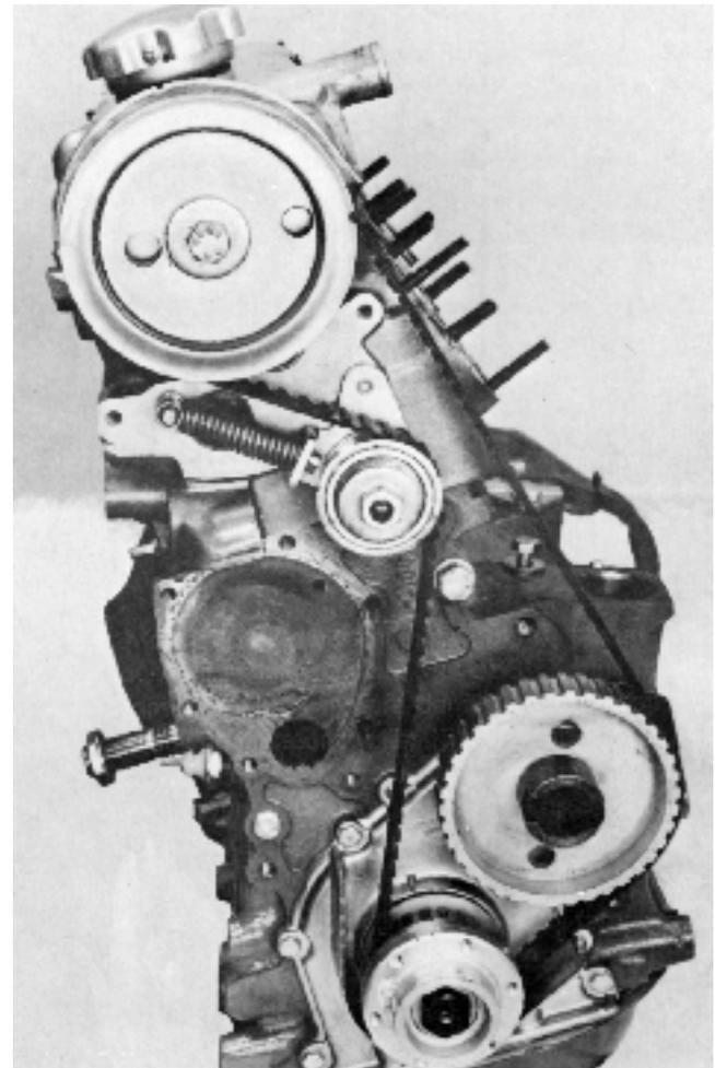
**131.** Refit the crankshaft pulley on the carrier.
