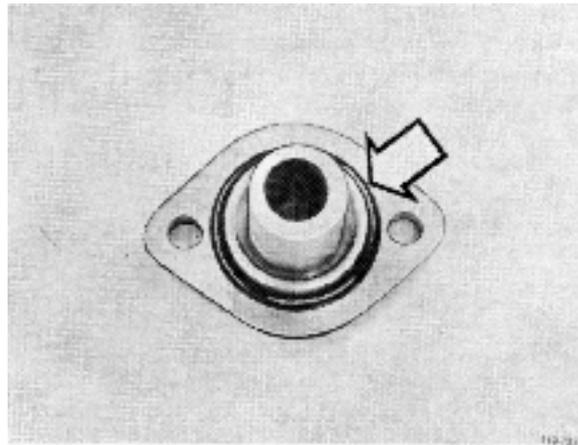
**132.** Fit the oil pump drive. It is possible that the crankshaft (intermediate shaft) may need to be turned somewhat so that the oil pump drive engages.
