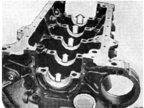
62. Note that there are markings for the main bearing caps. The bearing caps are marked 1–5 from the transmission side. Remove the main bearing caps.
