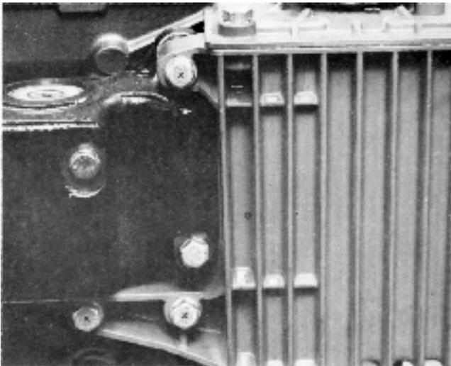
12. Unscrew the oil filter. Use tool 999 2903 or push a screwdriver through the filter and work it loose. NOTE! Be careful not to spill oil.
