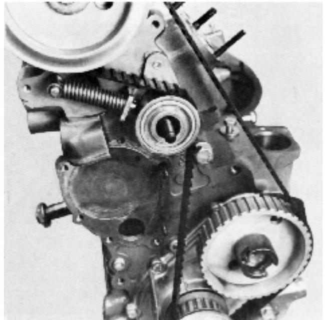
21. Slacken the belt by depressing the roller against the spring pressure. Lock the spring by inserting a 3 mm (0.118") pin (e.g. a drill) in the hole on the pressure pin.
