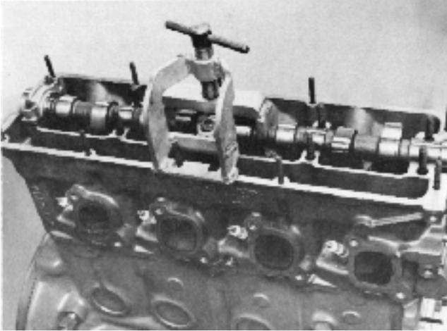
112. Lubricate the camshaft seal's rubber lip and fit it on the camshaft. Be careful so that the rubber lip is not damaged by the sharp edge when fitting it. Fit the sealing ring so that a new wear surface against the camshaft is obtained.
