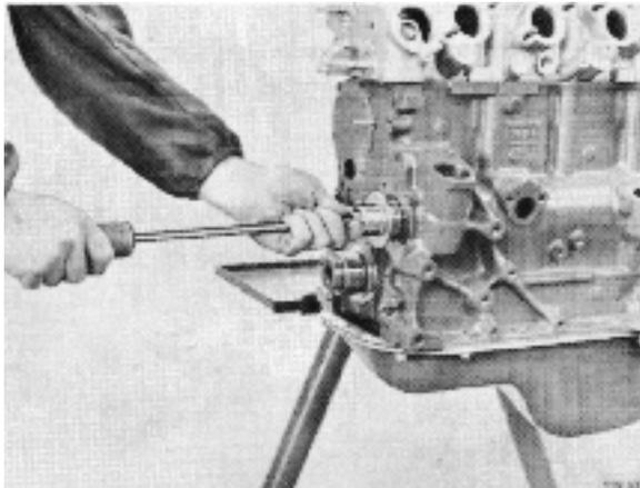
117. Fit the front sealing flange (and positioning plate) with a new gasket. The tightening torque is 10 Nm (1.0 kpm) (8.0 lbf. ft.). Then torque tighten the screws for the sump. The tightening torque is 10 Nm (1.0 kpm) (8.0 lbf.ft.).
