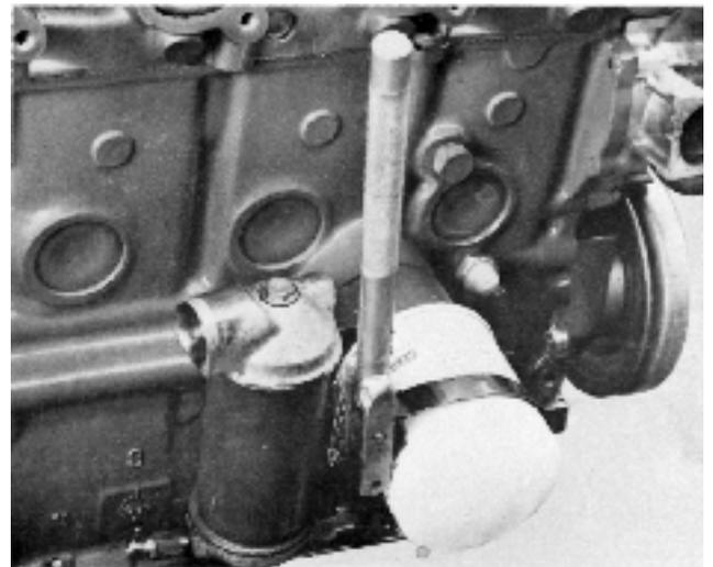
13. Remove the nut (1) and remove the oil cooler. Only AQ145. Spanner width = 28 mm. Remove the oil pressure
