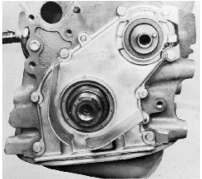
26. Remove the key and pull off the pulley and the inner guideplate from the crankshaft.
