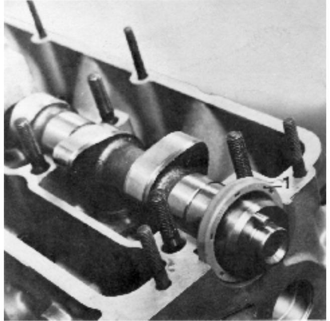
34. Fit tool 999 5021 on the camshaft. Use the bearing cap's nuts. The camshaft is held in position with the tool. Undo the other four camshaft bearing caps.
