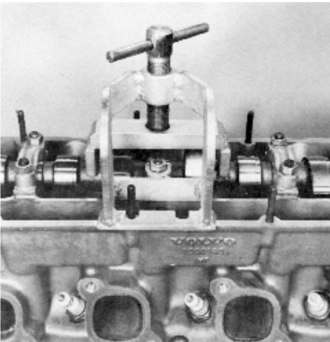
36. Remove the screws in the cylinder head. Use hexagonal socket key 10 mm. Lift away the cylinder head and remove the gasket. Remove the spark plugs.
