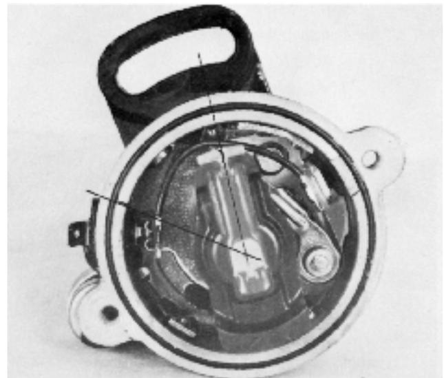
151. Press the distributor into position in the crankcase and check that the line on the rotor and the line on the distributor housing are opposite each other. Tighten the distributor in this position.
