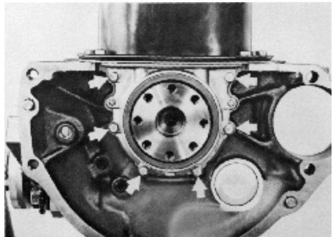
53. Remove the locking ring for the bearing on the input shaft.
