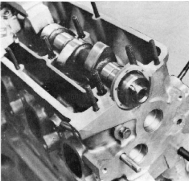
113. Oil and lay the other three bearing caps in position and fit the nuts for the four bearing caps. Tighten them somewhat NOTE! The forward bearing cap's surface against the cylinder head **is to be painted with sealing fluid** before it is fitted. Make sure that the seals fit correctly before the front bearing cap is tightened. Then remove the tool.
