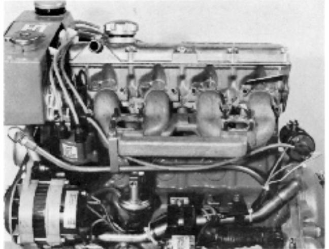
2. Remove the air filters (1), the fuel pipe (2) between the feed pump and the carburetors and unscrew the carburetors from the induction pipe. AQ125 has only one carburetor.
