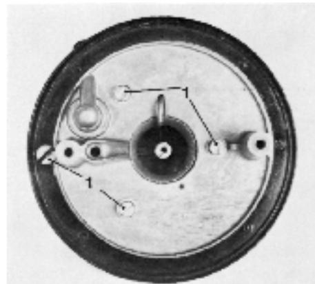
90. Remove the gasket (1) and disassemble the needle valve (2). Check that the needle valve does not bind or is worn (does not seal). Replace if necessary.
