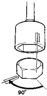
Tightening using both a torque setting and a protractor angle requires that first the recommended torque is applied using a torque wrench and then the recommended angle is added according to the protractor scale. Example: a 90° protractor tightening means that the joint is tightened a further 1/4 turn in one operation after the stated tightening torque has been applied.
