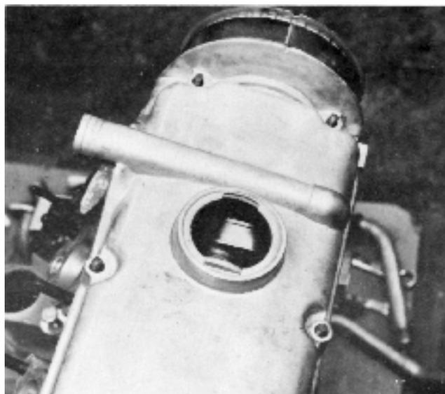
150. Turn the rotor so that the line on it is at 60° from the line on the distributor.
